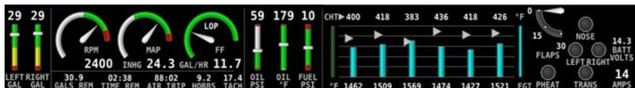
Figure 192: Example of an ENGINE BOTTOM BAND Page layout for single-engine monitoring.
