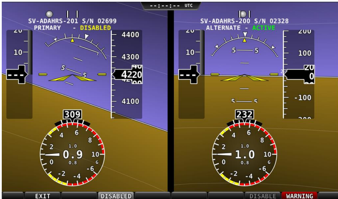
Figure 87: ADAHRS cross-check comparison (one ADAHRS disabled).
