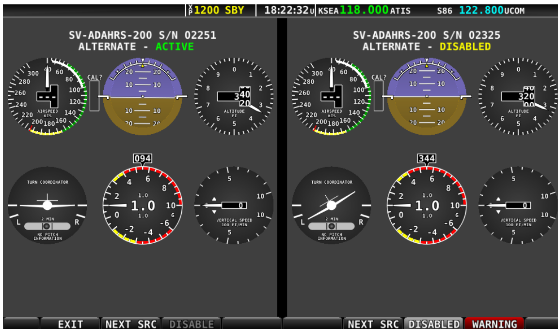
Figure 88: ADAHRS cross-check comparison (Six Pack presentation).
