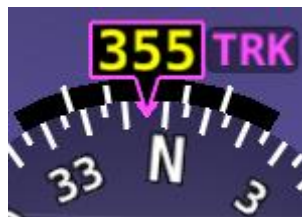
Figure 41: GPS Track substitute for Magnetic Heading indicator
