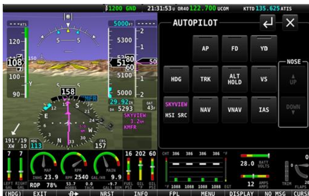
Figure 234: AUTOPILOT Page – Expert Control Scheme
