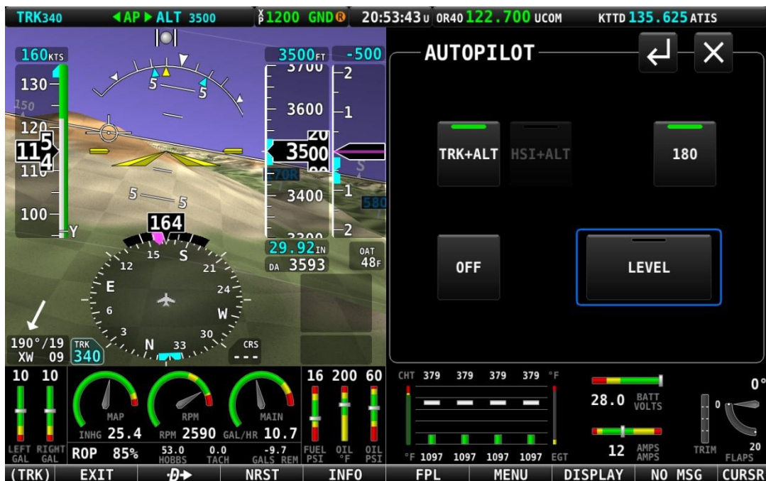
Figure 230: 180° Mode is engaged; turn is not yet complete.
