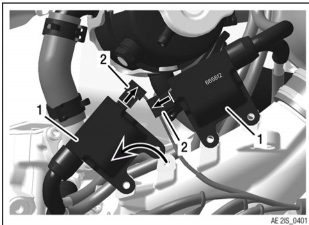
Figure 15.12: TYPICAL, for blade receptacle (male) connectors
