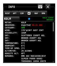
Figure 184: METAR - decoded
