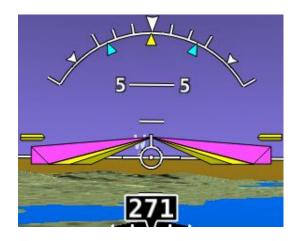
Figure 231: Single Cue / Inverted-V with Autopilot servos engaged.
