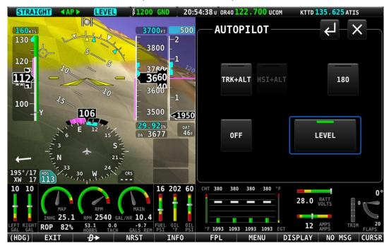
Figure 226: LEVEL Mode is engaged
