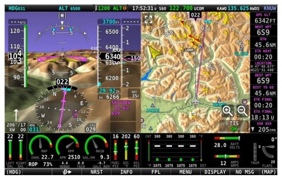
Figure 64: SkyView HDX Synthetic Vision - Normal View
