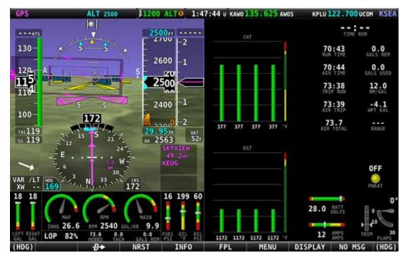
Figure 16: 50% PFD / 50% ENGINE with ENGINE BOTTOM BAND
