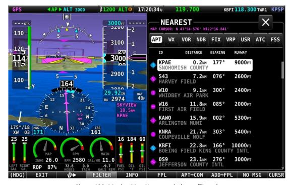
Figure 139: Moving Map Nearest window – filtered
