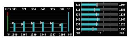
Figure 196 – Example of Combined CHT/EGT Gauge (Vertical and Horizontal Styles)
