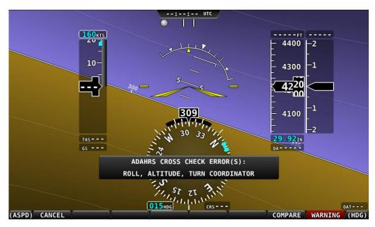
Figure 87: ADAHRS cross-checking disagreement.
