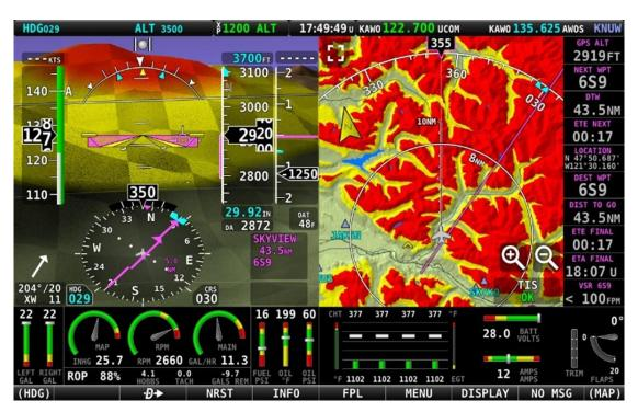
Figure 65: SkyView HDX Synthetic Vision - Terrain Alert
