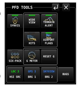
Figure 51: Bearing Pointer selector on PFD TOOLS page
