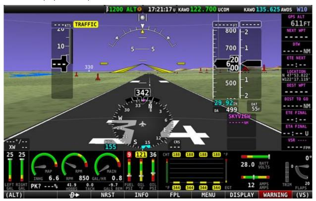
Figure 4: Displaying Main Menu Bar at bottom of the screen.
