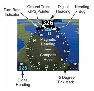
Figure 40: Magnetic Heading indicator / Directional Gyro
