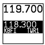
With a valid Com frequency highlighted, (25kHz frequency on the SV-COM-760, -T25, -425 and 8.33kHz on the SV-COM-T8) press the TUNE COM button to send the frequency to the standby frequency:
