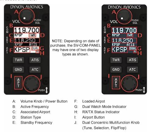
Figure 239: Com Radio Control Panel
