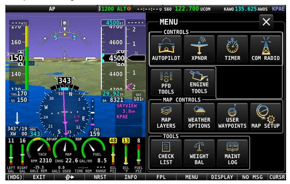
Figure 18: ENGINE BOTTOM BAND partially over-written by MENU Page.
