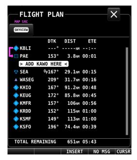
Figure 168: Flight Plan Waypoint insertion
