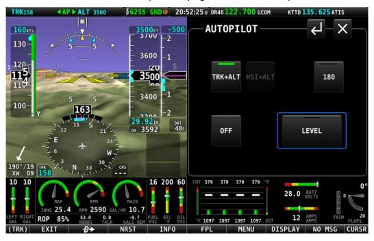
Figure 223: TRK+ALT mode is engaged.
