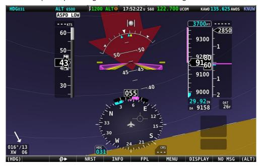
Figure 74: Extreme Pitch warning indicator arrows
