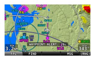
Figure 158: Flight Plan alert messages
