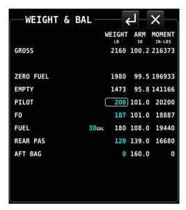
Figure 244: Weight and Balance calculator
