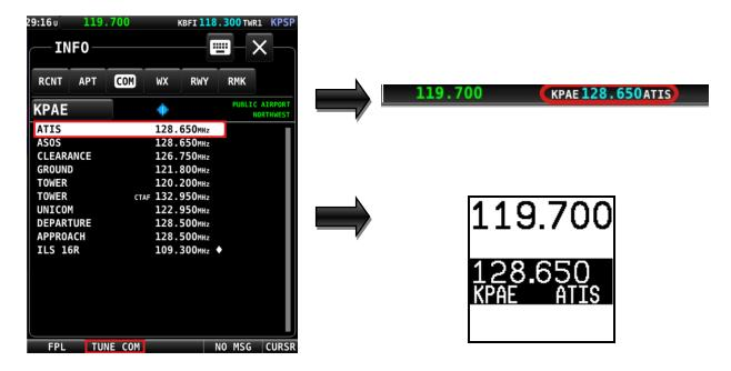
Press the dual concentric knob on the control panel to flip/flop the chosen frequency from the standby frequency to the active frequency.
