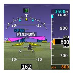
Figure 38: MIN Bug and "MINIMUMS" alert
