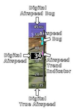
Figure 33: Airspeed Indicator example
