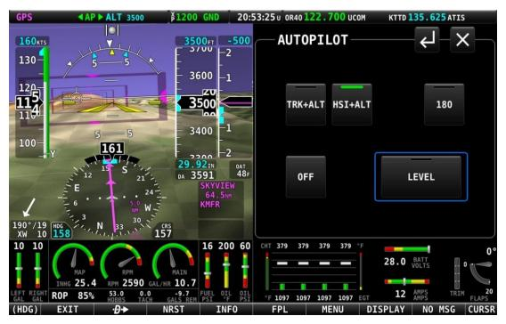
Figure 224: HSI+ALT Mode is engaged.
