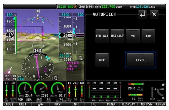
Figure 222: AUTOPILOT Page - Simplified Control Scheme
