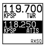
The squelch setting, which determines how strong a radio transmission must be before the radio receives it, is configured during setup. See the *SkyView System Installation Guide* or the *SkyView HDX System Installation Manual (Certified)* for instructions on adjusting this parameter.
