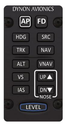
Figure 238: SkyView Autopilot Control Panel
