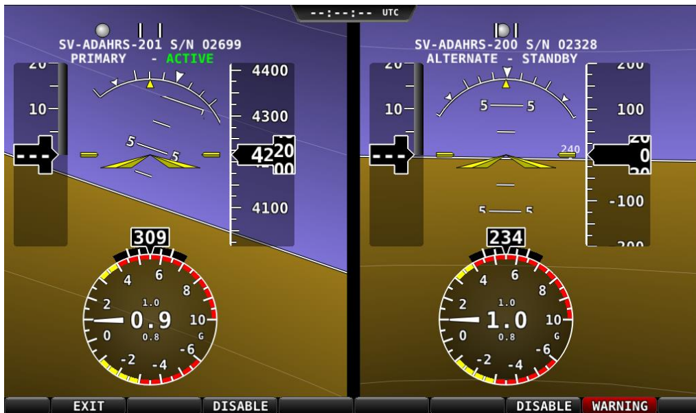
Figure 56 – ADAHRS Cross-Check Comparison
