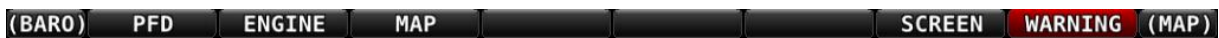
Figure 235 - Message Notification Area above button 8 (2nd from right), showing a Warning Notification
