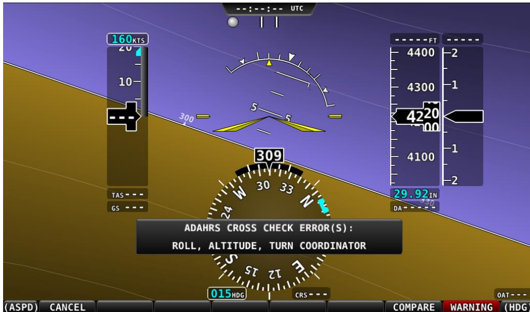
Figure 55 – ADAHRS Cross-Checking Disagreement
