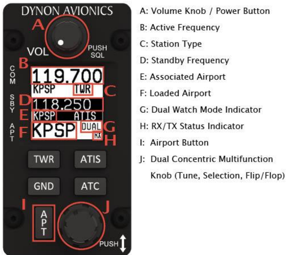
Figure 231 – COM Radio Control Panel
