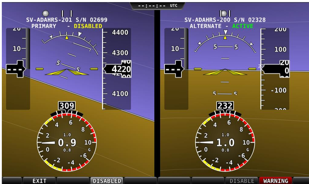
Figure 57 – ADAHRS Cross-Check Comparison (one ADAHRS disabled)
